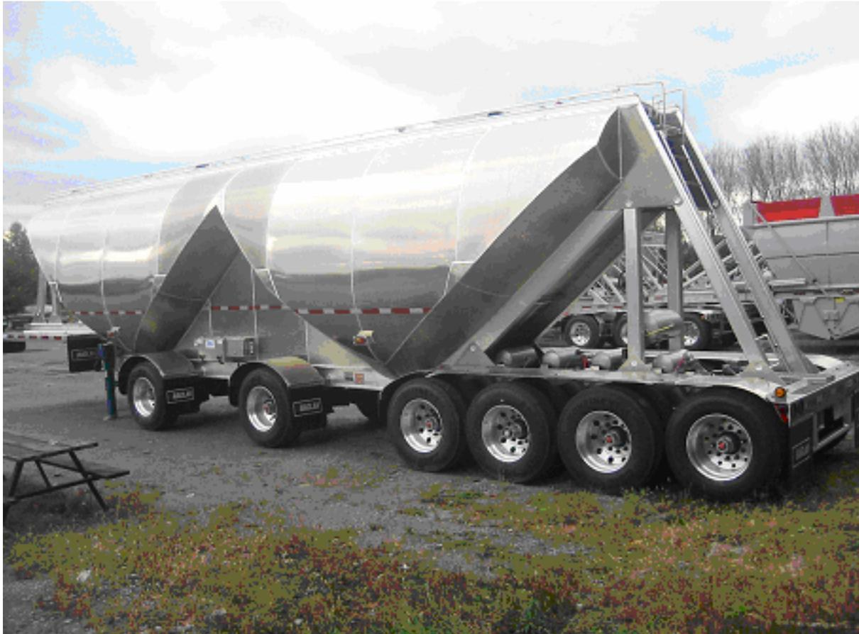
From Raglan Industries. *Semi trailer made after customers specification. The number of axles and the close spacing is to utilize the GVM limit.*
