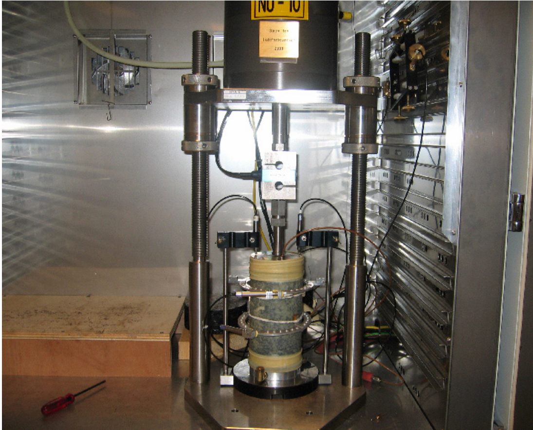
Figure 6: Test setup in the modified NAT
