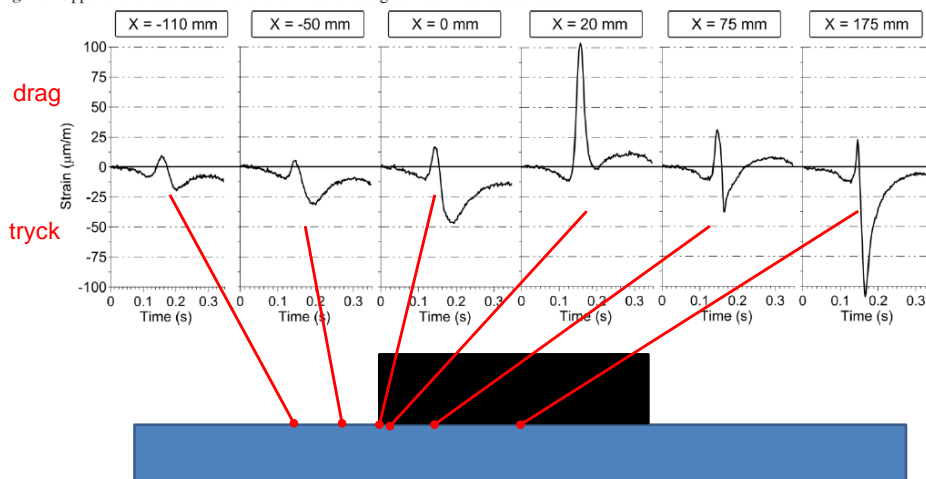
Fig. 10. Upper transversal strain evolution near the edge of the wide base tires.
