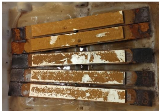
Steel-FRP adhesive joints after one year of immersion in salt water to be tested for evaluation of strength and stiffness degradation
