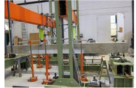
Research on Strengthening of concrete beams with pre-stressed CFRP laminates at Chalmers
